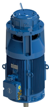
Three-phase asynchronous motor in non-ventilated version with electromagnetic spring-set brake and protected hollow shaft incremental encoder between motor housing and brake, type of protection IP 56
